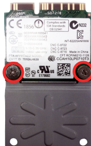
Join the WiFi module and the “mini half bracket” by using two screws.
