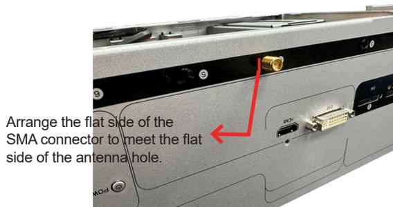
11. Mount the washer first and then the nut to the SMA connector. Make sure the nut is tightened.
