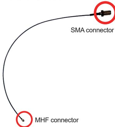
5. Connect the RF antenna’s MHF connector to the Wi-Fi module’s main connector marked 0. If you are going to connect a secondary antenna, connect it to the connector marked 1.
