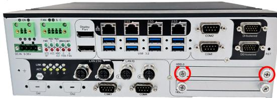
2. For the 1st storage bracket, slide the HDD/SSD storage device into the bracket.
