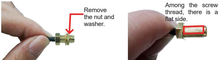
10. Pull the SMA connector through the above mentioned antenna hole. Note to meet the aforesaid flattened side with the antenna hole's flat side.
