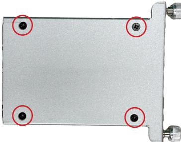
4. If you are going to install the 2nd HDD/SSD storage device, slide the storage device into the bracket and fix it in place in the same way.
