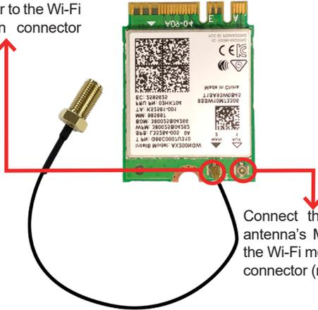
Connect the secondary RF antenna's MHF connector to the Wi-Fi module's secondary connector (marked 1)
