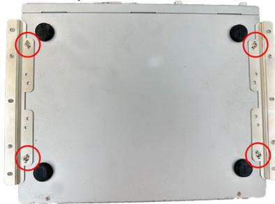
2. When the bracket is attached, the computer can be hung on the wall as the way you want. The wall mount bracket dimension is shown as below:
