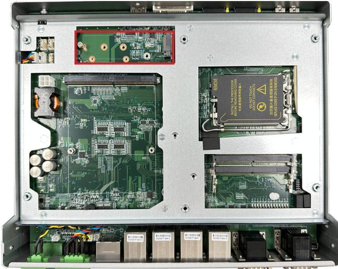
2. Insert the M.2 module into the socket by aligning the notch on the module with the small slot on the M.2 socket.
