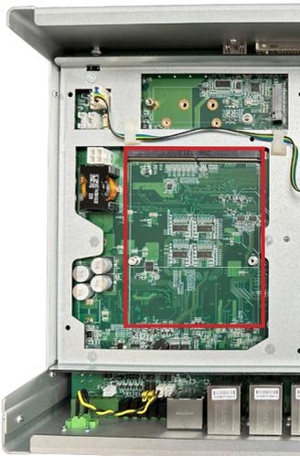
3. Install the graphic card into the computer correctly.
