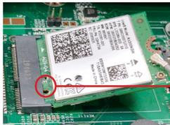
The module's key notch should meet the connector's break.
