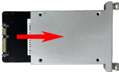
3. Fix the storage device in place by fastening the four screws of the bracket.
