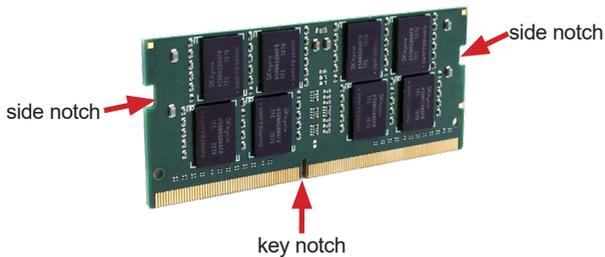
The computer has two 262-pin DDR5 SO-DIMM sockets that each socket support up to 64 GB maximum system memory. To install a memory module:
