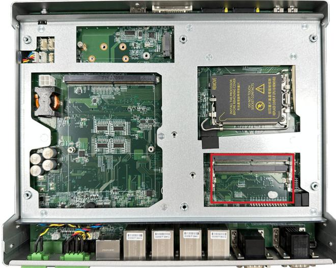
3. Align the notch on the memory module with the key in the module socket.
