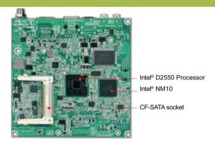
NANO-5050 adopts latest Intel® Atom™ D2550 CPU and NM10 chipset which is for the low power compact size system. The new architecture integrates the 3D graphics engine and memory controller. It's suitable for Medical and Networking applications.
