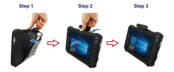
Position the Tablet PC into the docking and insert the tablet
